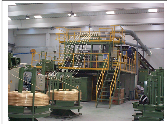
Rautomead RS 2500 in production of 8mm binary brass
