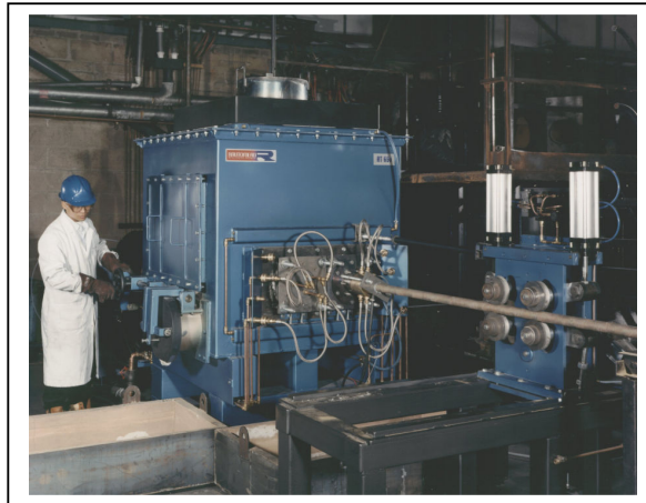
Rautomead RT 650 continuous casting machine (70 litre crucible capacity, 275 kgs per hour)
