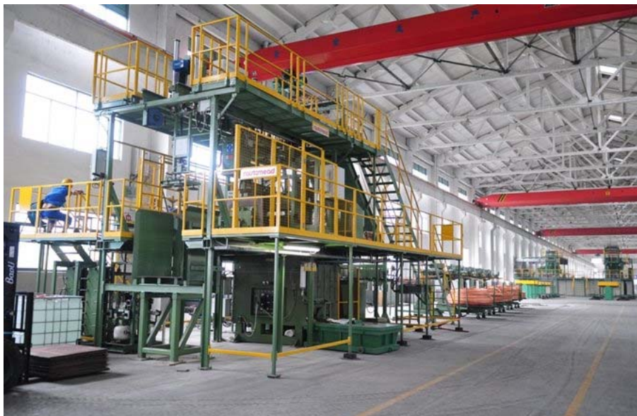
Fig. 9 Rautomead RS 3000/5-Cu-Mg Casting Machine
